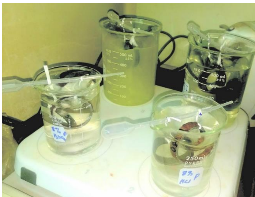
Figure 2. Tube samples exposed to acid to determine effectiveness of inhibitor with organic additives.
