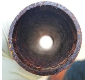
Figure 4b. Cleaned tube following 7.5 hrs treatment including re-batching.
